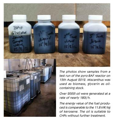
The Pyro-BAF-Technologie is an efficient two-stage process for decentralized energy production to generate engine-suited fuels from biomass in combination with oil-containing residue for use in combined heat and power plants (see reverse).
